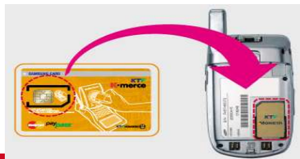
Provision Credit Card Application into the UICC/SIM
